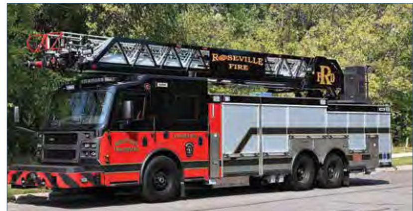
Roseville's fire ladder can reach up to 109 feet and is able to reach the ninth or tenth story of a building
