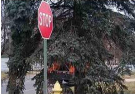
Tree branches obstructing vision at traffic control sign
